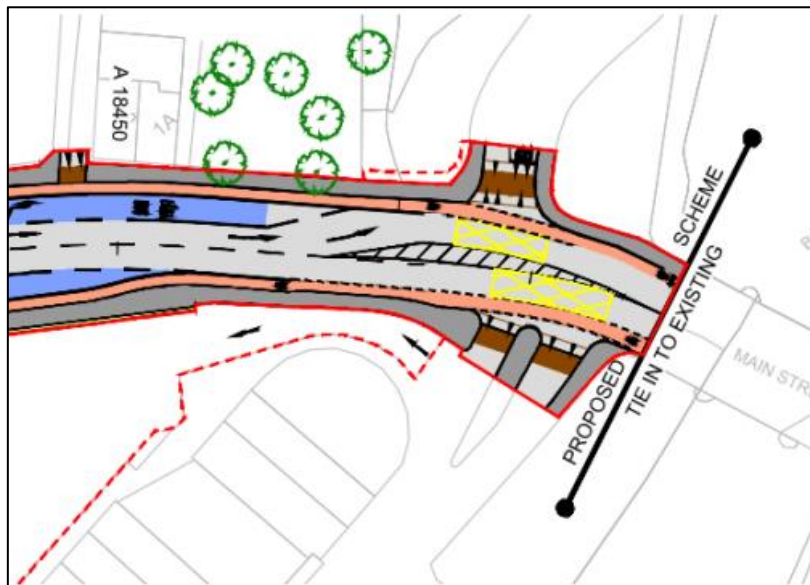
Figure 2.207: Extract from General Arrangement Drawings showing the Proposed Scheme design tie-in to the Existing Design (Sheet 52)
