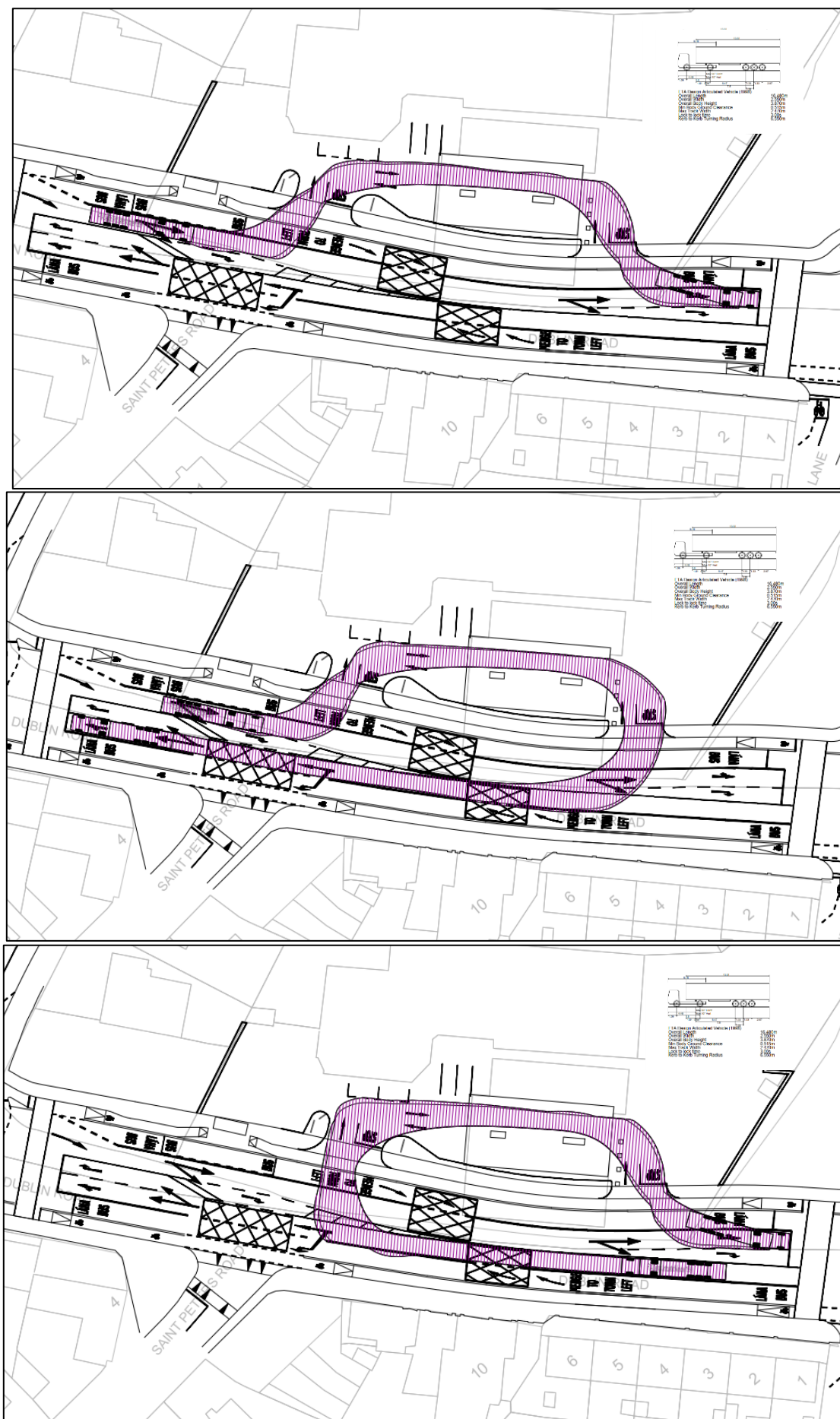
Figure 2.129: HGV Swept Path Analysis at Circle K, Dublin Road, Bray
